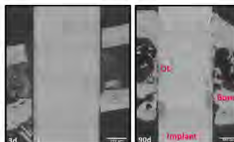
Figure 1 Overview of the degradation and bone formation of the WE43 implants after 3 and 90 days using synchrotron radiation micro-CT.
