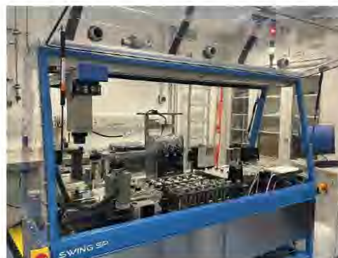
Fig. 1: Robotic testing platform at Institute of Surface Science, Helmholtz-Zentrum Hereon for high-throughput testing of metallic materials in complex aqueous electrolytes.
