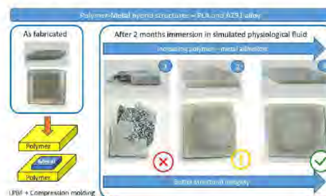
Fig. 1: Polymer-metal hybrid structures.
