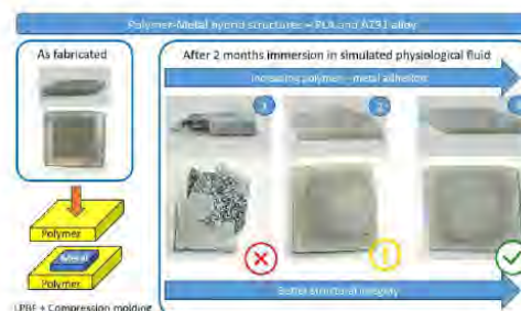
Fig. 1: Polymer-metal hybrid structures.
