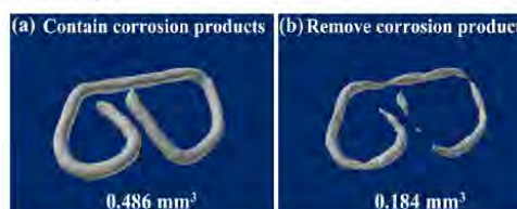
Fig. 2: In vivo degradation morphology of Zn-based staples implanted in stomach of Beagles for 12 months.
