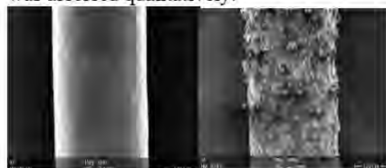
Fig. 1: Silk fibroin coated wire (Method: EPD; Solvent System: DES (left) and IL (right)).
